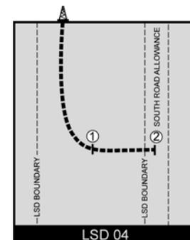
If drill hole (1) encounters an oil sands pool, an alpha character (AA to HZ) will be assigned to the local exception code. The characters “I” and “O” are not used (e.g., AA/04-08-070-03W4/0).
