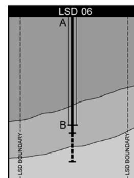
5) Directionally drilled well projected to bottom in a specified legal location
