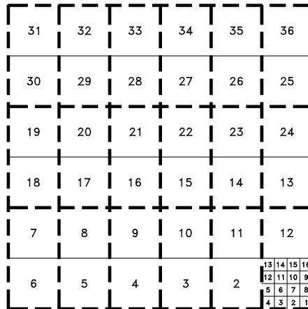
The darkened lines above indicate road allowances. A well that terminates (i.e., TD) in a road allowance is referenced either south (S) or west (W) of the legal subdivision indicated in the unique well identifier.
